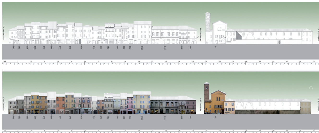
Fig. 5. The rectified images and the graphic drawing of the façade of Via Bixio: second part.
