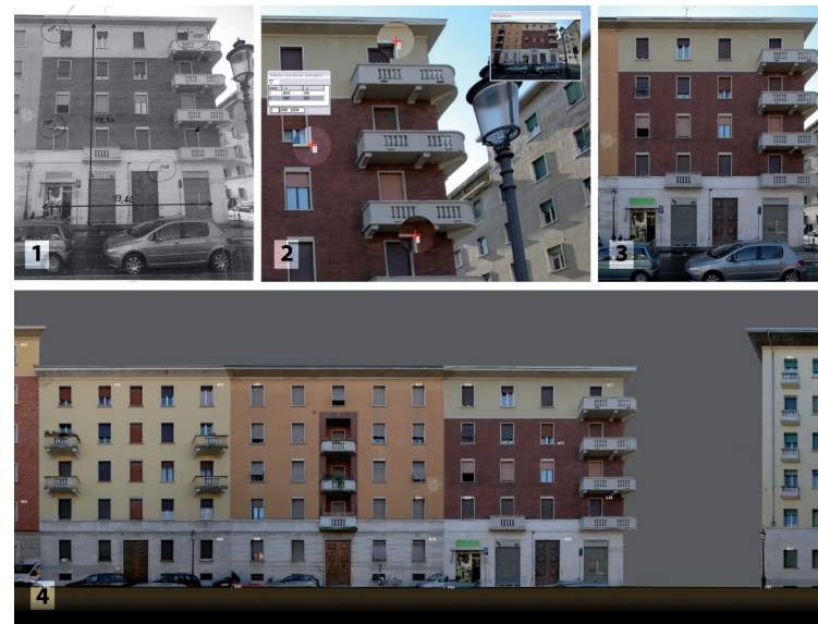
Fig. 3. The four steps provided by the methodology used for the survey of urban curtains, defined as "monoscopic photogrammetric survey": 1 survey on the street with total station, 2 identification of recorded points on the photographic image, 3 straight and scaled the photo, 4 photomosaic of the streets façade.
