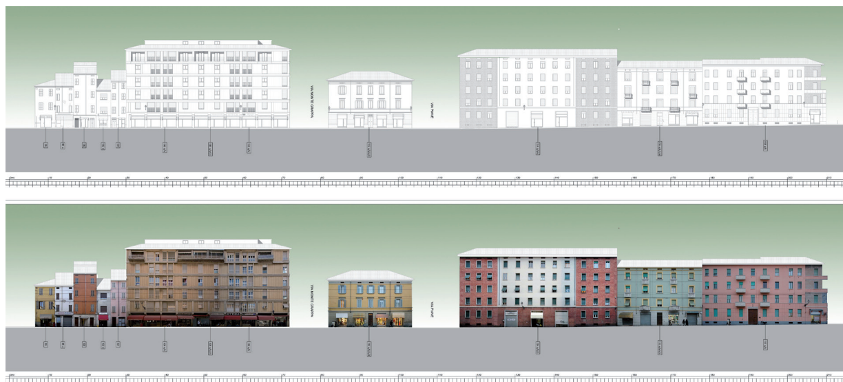
Fig. 6. The rectified images and the graphic drawing of the façade of Via Bixio: third part.
