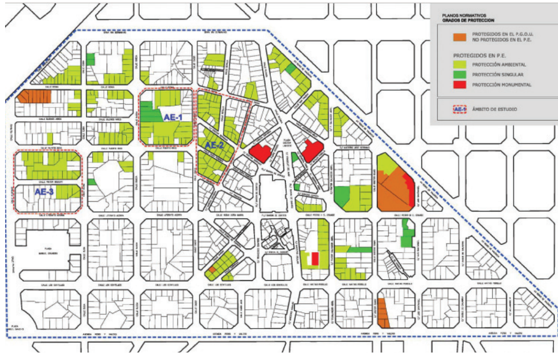
Figure 2 This map represents the degrees of protection in Ruzafa. Environmental, singular and monumental protection. A big quantity of buildings in the historic core are protected, and the interventions must respect the values of the buildings. Jimenez, C. (2012). Research project: Proposed Assessment Methodology and Historic Neighborhood Building typological classification. For BRCC02 (Ruzafa neighborhood almost zero energy consumption). University Politechnic of Valencia. p.p. 214
