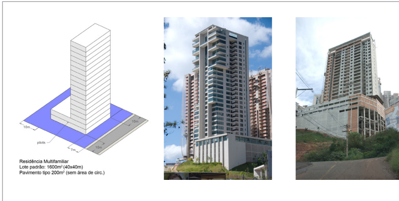
Figure 12 – Standard template pattern, permitted in 2007’s Director Plan (to the right) and the trays generate by blind walls (to the left). Source: Zyngier, 2012 (to the right) and personal archive Moura, 2011 (to the left).
